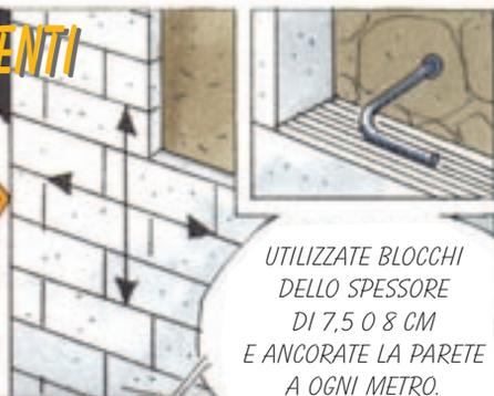
UTILIZZATE BLOCCHI DELLO SPESSORE DI 7,5 O 8 CM E ANCORATE LA PARETE A OGNI METRO.
